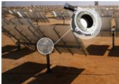
Figure 2. BrightSource's current twofacet pedestal heliostat design; Source: Roadmap to Advance Heliostat Technologies for Concentrating Solar-Thermal Power , link to reference?
