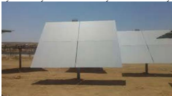
Figure 5. Wireless BrightSource heliostat at Ashalim with top-mounted PV panel; Source: Roadmap to Advance Heliostat Technologies for Concentrating Solar-Thermal Power, Source : https://www.nrel.gov/docs/fy22osti/83041.pdf
